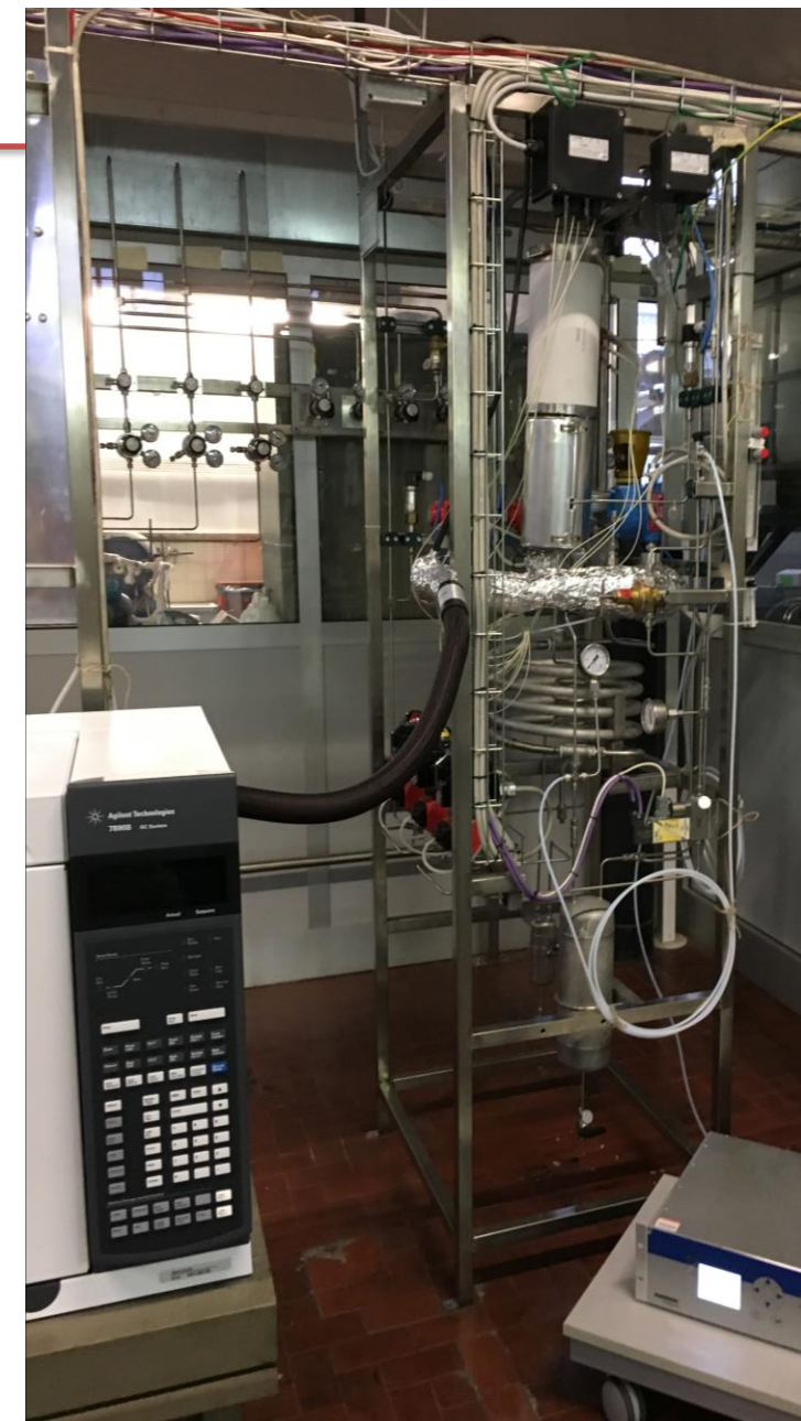
Production of synthetic chemicals through CO 2 hydrogenation tests
